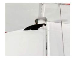
9 Take out the 4 ball joint connecting rods, install 1 of the 58.5mm on the left as well as the right wing. Next, install the 60.5mm on the rudder, and the 90.5mm on the elevator.
