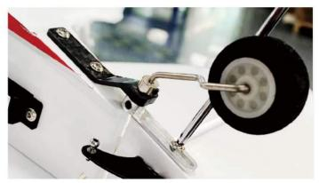
Take out the left and right wings and slide them on to the carbon fiber wing tubes. and tighten the M5 nylon screws. Then, place the fuselage bottom up and remove the screws at the bottom of the wings. If necessary, gently bend the tips of the wing supports so the ends are flush with the respective screw holes on the wings and fuselage. Be sure to align the large wing supports towards the leading edge of the wings, and the smaller ones towards the trailing edges.
