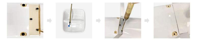
Take out the horizontal stabilizer and insert it face up into the slot in the tail of the fuselage, be sure to insert it fully. Insert the wing tubes into the front of the fuselage. Look forward from the rear of the fuselage to make sure that the horizontal stabilizer and wing tubes are parallel, and then use adequate glue on the gap to affix the horizontal stabilizer on the fuselage.
