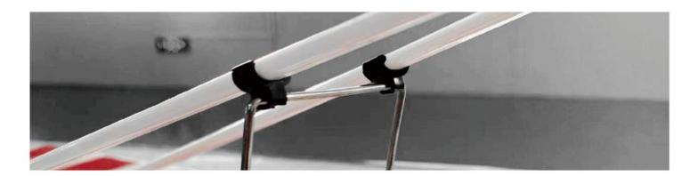
Insert the cable through the sleeve, and then thread the cable through the hole of the vertical stabilizer cable buckle, and then thread it back into the sleeve. After adjusting the tightness of the cable, use pliers to clamp the sleeve.
