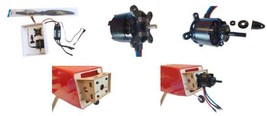
2. Flip over the fuselage and remove the front plate, this is where the speed controller can go and tie that in place, connect up the phase wires, recommend you put some electrical tape around the phase wires so that there's no danger of them coming disconnected from the wires from the speed controlle, close up the back plate.
