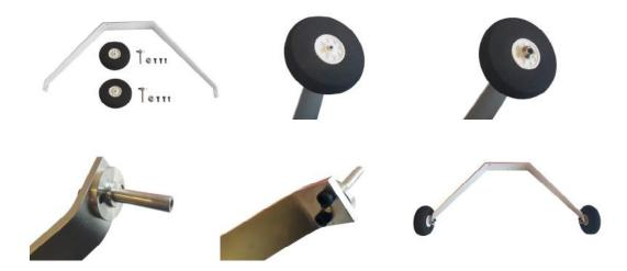
2. Underneath the fuselage, undo three bolts, then attach the landing gear
