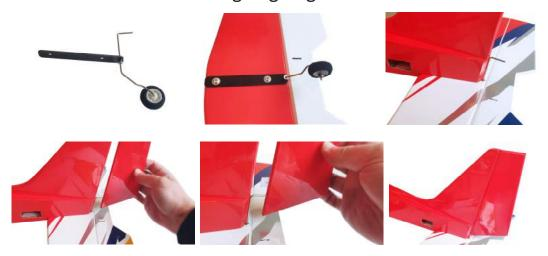
3. Dry fit the rudder, then put the fuselage on its side and drip in just a small number of drops of thin CA glue.
